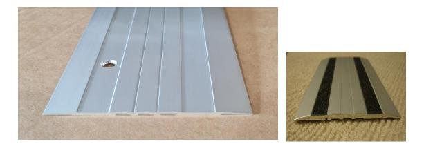
The ST 100 CJ trim is a 100mm slim line clear anodised aluminium cover plate designed to go over the top of resilient floor coverings. 3.5mm in height.
