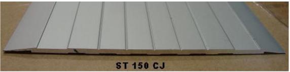
The ST 150 CJ trim is a 150mm slim line clear anodised aluminium cover plate designed to go over the top of resilient floor coverings. 3.5mm in height.
