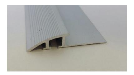
The ST 22-5 CT trim is designed to be fixed directly to the subfloor for use with a 6-7mm soft floor covering inserted into the 5mm cutout leaving 20.32mm of exposed aluminium.
