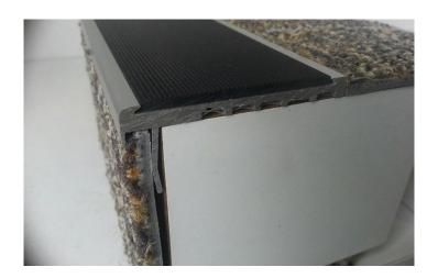
The ST 61-6 CC nosing is 61mm on the tread with a 50mm insert and a 10mm visible riser, it is suitable for carpet tiles and 6mm direct stick carpet.
