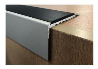
The ST 74 LN (long nose) clear anodised aluminium stair nosing is 75mm on the tread with a 50mm pvc insert and has a 45mm external riser.
