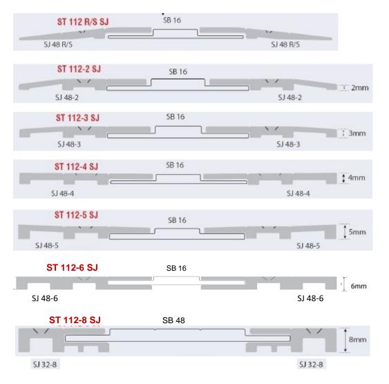
The Spacer Bar can be changed to one of the following to alter the width. i.e 2 x SJ 48-4 End Pieces &  $1 \times SB 96 = 192$ mm plus a 3mm gap.
