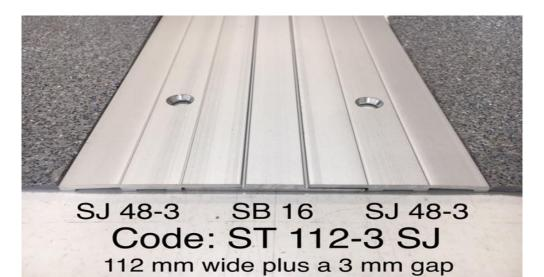
**DESCRIPTION:** ALUMINIUM 3 PART SLIP JOINT AVAILABLE IN VAROIUS WIDTHS. IT SHOULD BE FITTED WITH A **3MM GAP TO ALLOW FOR CONTRACTION** AND ALLOWS FOR **12MM OF EXPANSION**. AVAILABLE WITH Reducing (R/S), 2mm, 3mm, 4mm, 5mm, 6mm or 8mm END PIECES. The Spacer Bars are available in 16mm, 32mm, 48mm, 96mm & 128mm Only the 2 end pieces are screw fixed.
