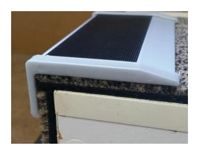
The ST 74 clear anodised aluminium stair nosing is 75mm on the tread with a 50mm pvc insert and a 35mm riser.
